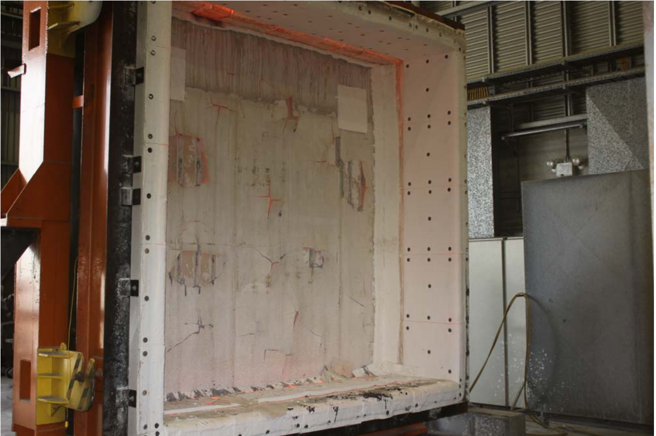
PHOTOGRAPH 10 – EXPOSED FACE OF THE SPECIMEN AFTER THE CONCLUSION OF TESTING
