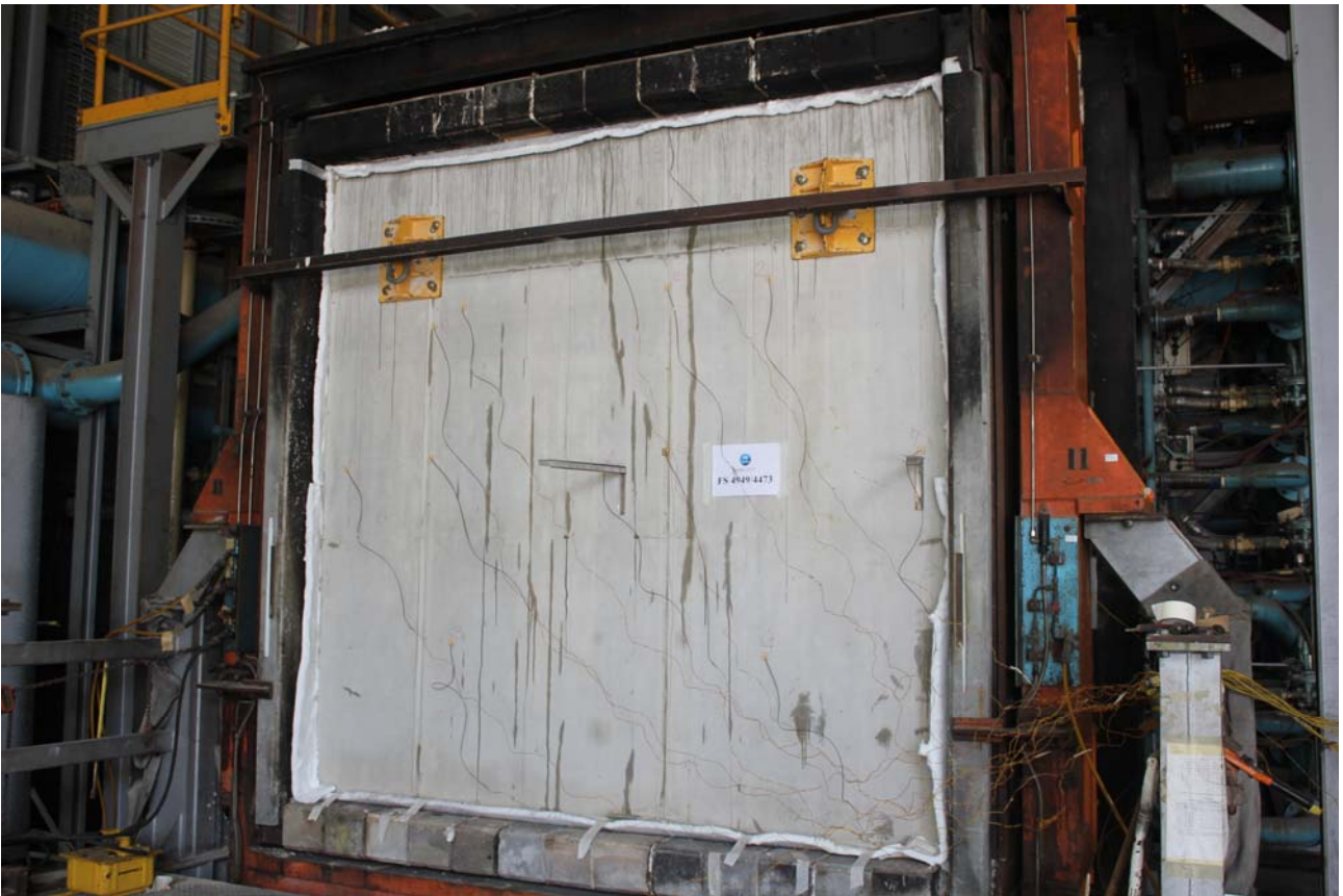
PHOTOGRAPH 7 – SPECIMEN AT 120 MINUTES INTO THE TEST
